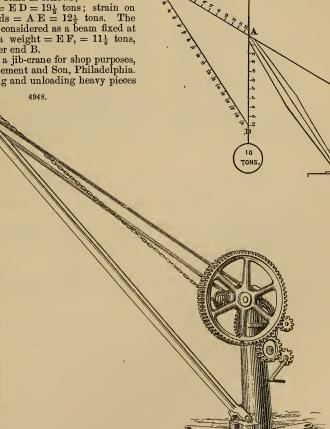
from planers and other tools, or for general lifting work. The machinery, including the jib, is all mounted on a strong metal post revolving on a stud attached to and supported by radial feet which are bolted to the foundation.
